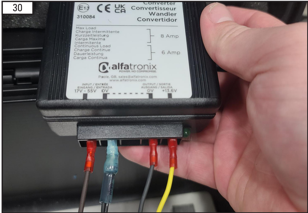
Before pushing in the switch to activate the system ensure the converter is connected as shown above.
