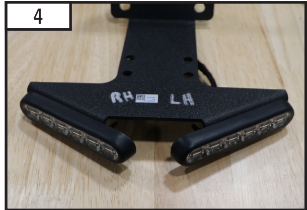
4 Grab one left and one right mpower light. Mount the lights to the appropriate side of the siren speaker bracket called out in the image.
