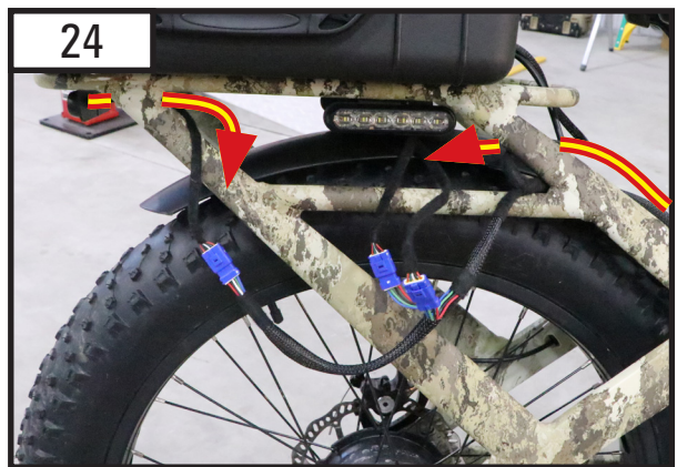
24 Connect the rear lights making sure the longest blue connector is attached to the rear facing light. Ensure the cables are ran on the inner side of the bike frame so they are protected.
