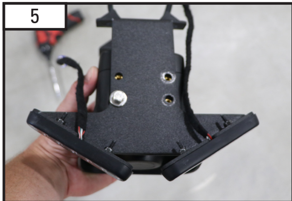
5 Now mount the siren speaker to the bracket, using the 4 bolts, 4 lock washers, and 4 washers provided in the siren speaker box.
