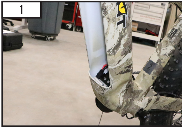
1 Remove the battery from the bike's lower frame.
