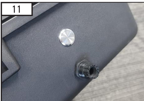
11 Install the switch in the upper hole and wire pass through grommet in the bottom hole.
