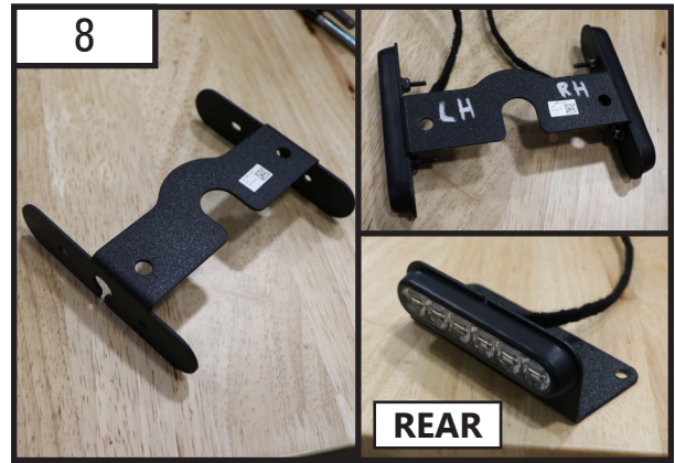
8 Grab rear brackets and mount the lights to the appropriate location called on the brackets in the image.
