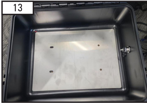
13 Place box on top of the rack, insert the internal reinforcement plate. Push bolts through the plate, box and rack with supplied hardware.
