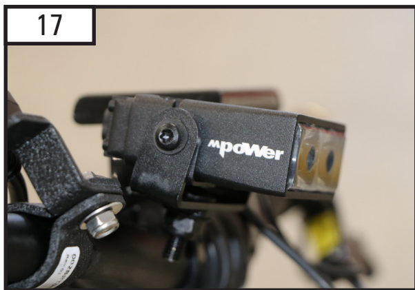
17 Mount 2x1 HPS to the right hand bracket with the bail bracket already installed. Use the hardware provided with the 2x1 HPS kit.
