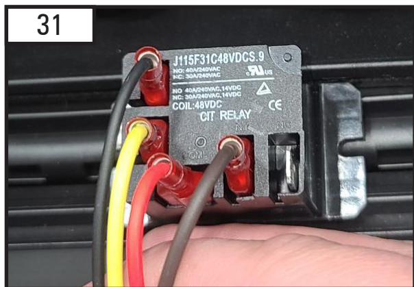
Before pushing in the switch to activate the system ensure the relay is connected as shown above.
