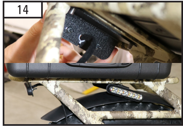
14 Line up light brackets and slide onto bolts. Tighten bolts once box is correctly aligned.
