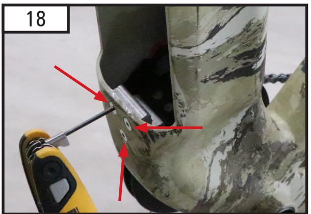
18 Remove the bikes 48v battery bottom mounting bolts (3x 3mm allen)
